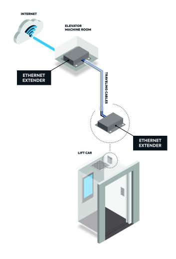
When it comes to installing the Ethernet extender in the elevator cabin, a useful location is inside the car operating panel, providing easy access for maintenance and troubleshooting. Additionally, this location helps to keep the Ethernet extender out of sight and secure from unauthorised access.
